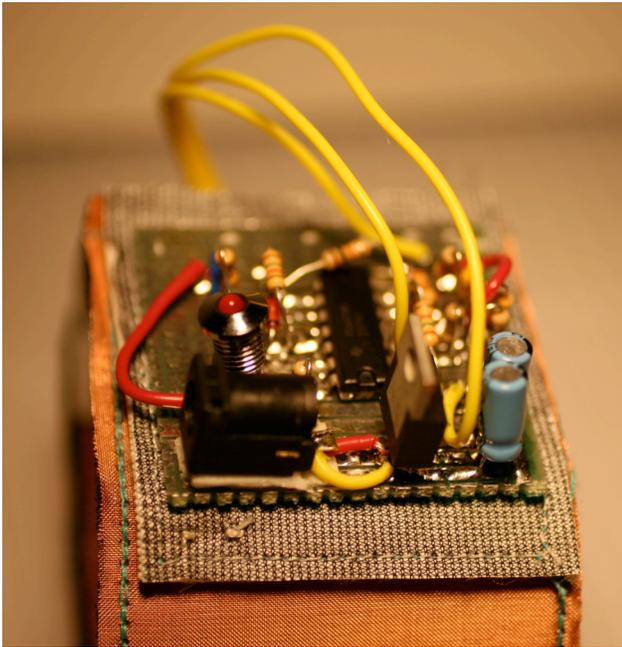
**Figure 2.** The prototype circuit on the EMF detector bracelet.
