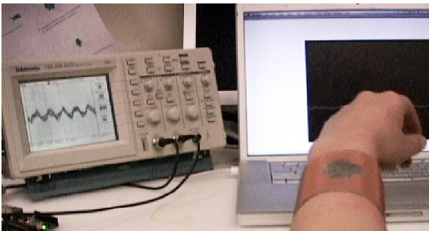
**Figure 3a.** The bracelet is located at 14 inches away from the display – the oscilloscope shows the front-end output.
