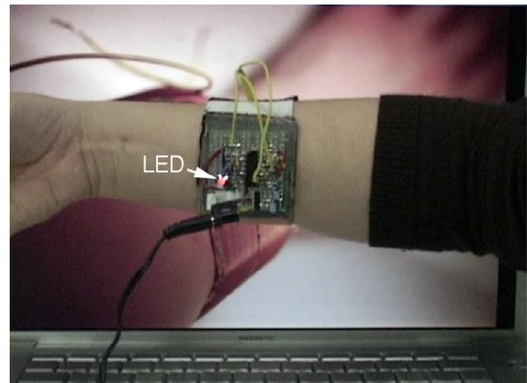
**Figure 4.** The battery-powered bracelet is at 1 inch away from the screen, where the feedback LED is fully illuminated.
